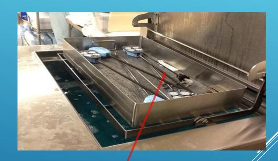
Hang test around perimeter or place flat in the basket for ultrasonic cleaners – do not obstruct test
