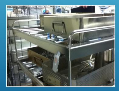
Hook the test around the perimeter of the rack, do not obstruct the spray arm movement
