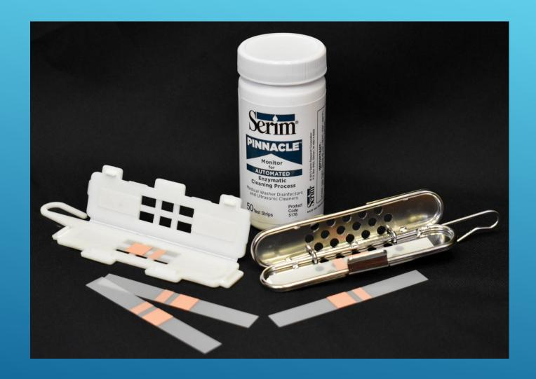
Both resin and stainless steel holders were improved in 2021 to provide a more robust cleaning challenge. All holders in this presentation can be used in both washerdisinfectors and ultrasonic cleaners
